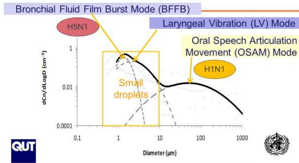
These conclusions were reached using a flow tunnel, which allowed for the measurement of the concentration of droplets and their size distribution in the
